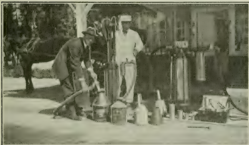
FIG. 226. Testing the accuracy of gasoline pumps. This branch of the work has increased to such an extent that it has necessitated the employment of several additional deputies.
